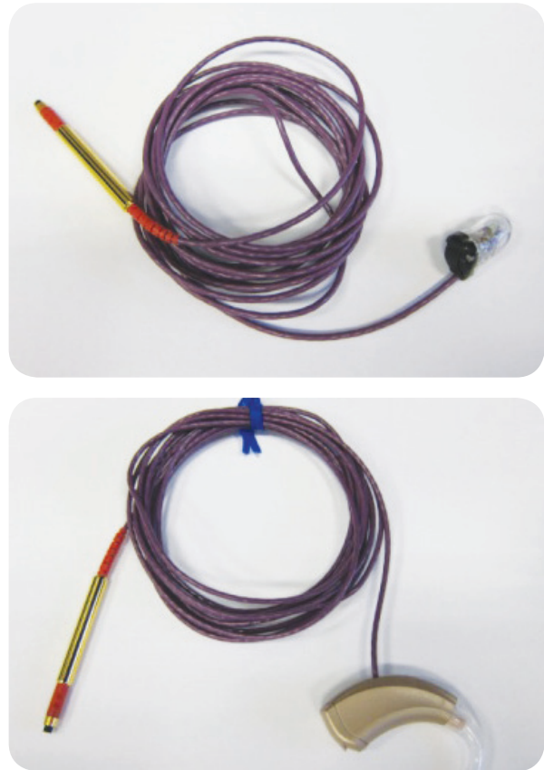
Figure 2. IIC and BTE hearing aids are shown. Each was specially prepared for recording; a cable has been attached to the hearing aid microphone for in situ audio recording.
