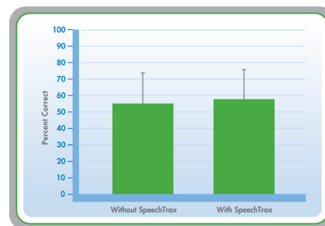
Figure 5. Percent correct on the nonsense syllable test (NST) with and without SpeechTrax digital noise reduction processing.
